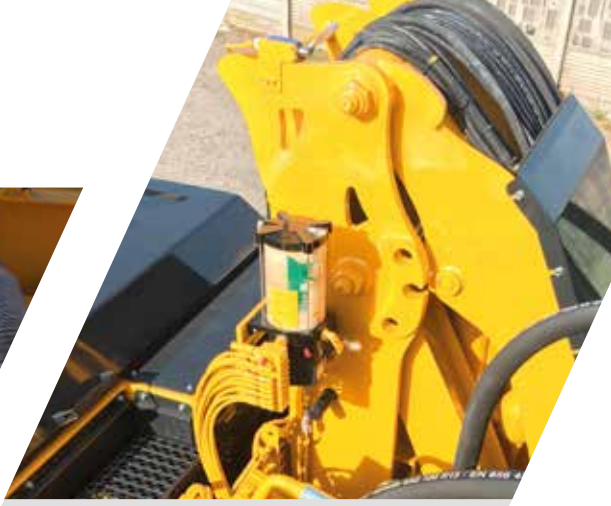
New scissor-type cab lifting system
